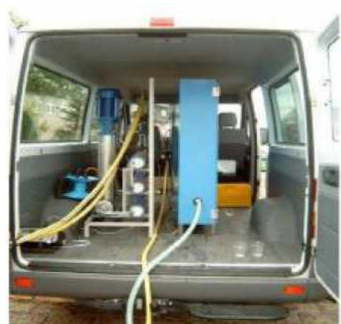
Small device for production of potable water, operates with solar energy, accomodated in small truck
