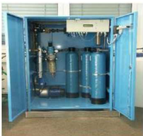
Small device for production of potable water, operates with solar energy, accomodated in small truck
